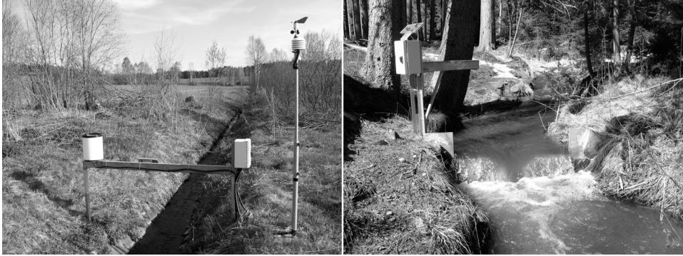
Fig. 3 – Meteorological station and water-level measure – The ZBY Brook (left), water-level measure – the TET Brook (right)
