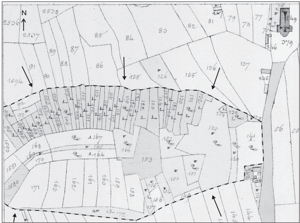
Fig. 9 – Map No. 0663-1-009 of the Stable Cadaster. The dormant landslide, see also Figure 8, can be easily delimited from the shape and the arrangement of the parcels and from the different land use. Source: Archive of the Czech Office for Surveying, Mapping and Cadaster.
